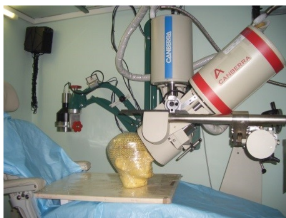
Measurement of Am-241 in a USTUR skull phantom with CIEMAT LE Ge detector. EURADOS Intercomparison
